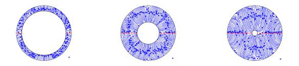
(a) Eletric field lines with b/a = 1.25 (b) Eletric field lines with b/a = 2.5 (c) Eletric field lines with b/a = 10
