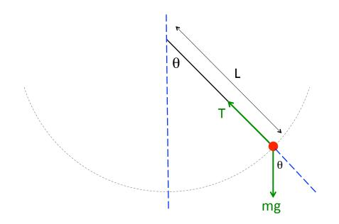
We can understand the motion by drawing a free-body diagram of the system and resolving the forces acting parallel and perpendicular to the rod. Since the particle moves on a circle, the forces in the radial direction must combine to provide the correct centripetal force,  $m\omega^2 L$ , where
