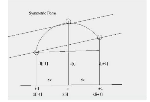
The following program (Derivative.cpp) reads a tabulated function from the input stream and calculates its numerical derivative using the three numerical forms, Forward, Backward, and Symmetric.
