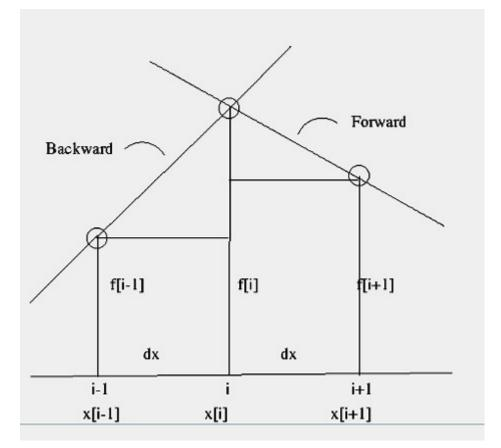
A low-order approach follows by using the points i and i + 1—the Forward formula. The Backward formula follows the same procedure but is based on the points i - 1 and i. Both formulae for the derivative at i yield the same slope in the limit  $\Delta x \to 0$ , as discussed in any calculus textbook. However the numerical approach always implies finite  $\Delta x$ , and therefore not so accurate results.
