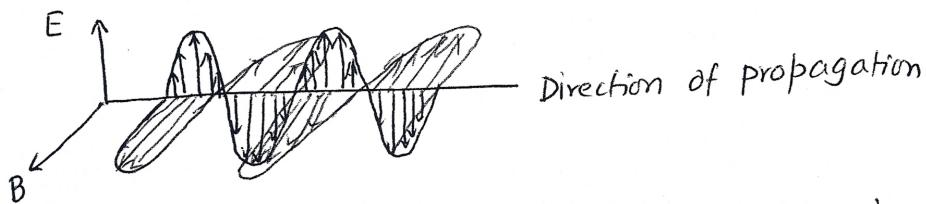
Maxwell equations (given below) show that a time varying magnetic field acts as a source of electric field and vice versa. These  $\vec{E}$  and  $\vec{B}$  fields sustain each other, forming an electromagnetic wave that propagates through space.
