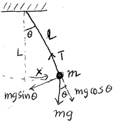
A simple pendulum consists of a point mass suspended by an inextensible weightless string. When pulled to one side and released, the pendulum executes SHM about the equilibrium position.
