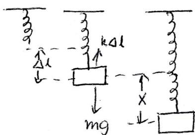
Motion of a suspended body from a vertical spring:
