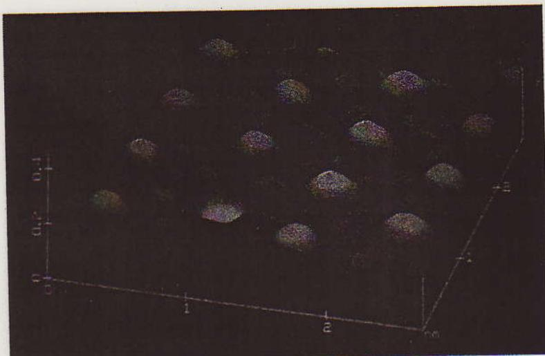
STM uses electron tunneling to create images of surfaces down to scale of individual atoms.
