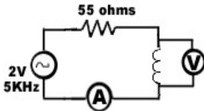
Notice that the AC voltmeter measures the voltage drop across the inductor, not across the entire circuit! Therefore the 55 ohm resistor does not affect our calculation of  $Z$ .
