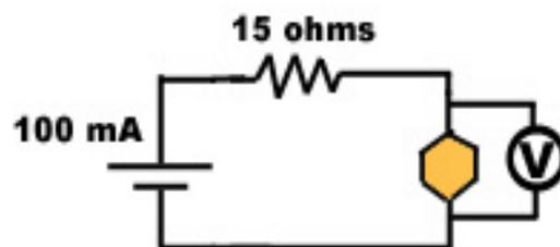
The equipment should be connected as shown: a DC power supply, 15-ohm resistor, and the **black wires** from the BSCCO sample are connected in series. (The hexagon in the diagram represents the BSCCO sample and the V is a high-precision voltmeter. The thermocouple leads are not shown because they are not part of the circuit.)
