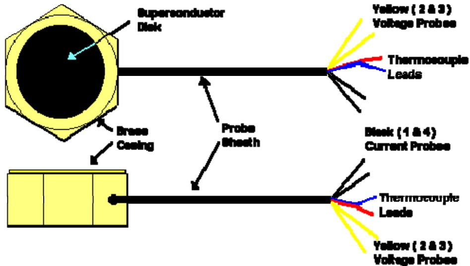
**Figure 2: The Superconducting Four-Point Probe**
