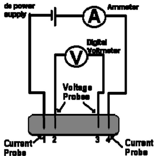
**Figure 2: Schematic of Four-Point Probe**
