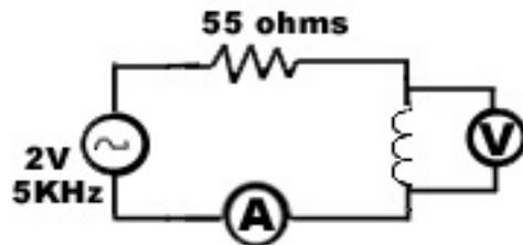
This experiment is very similar way to the first, except that the circuit now uses alternating current and the BSCCO sample has been replaced by an inductor with a YBCO core. The AC power supply, 55 ohm resistor, and another portable multimeter should be connected in series with the **black wires** from the inductor.
