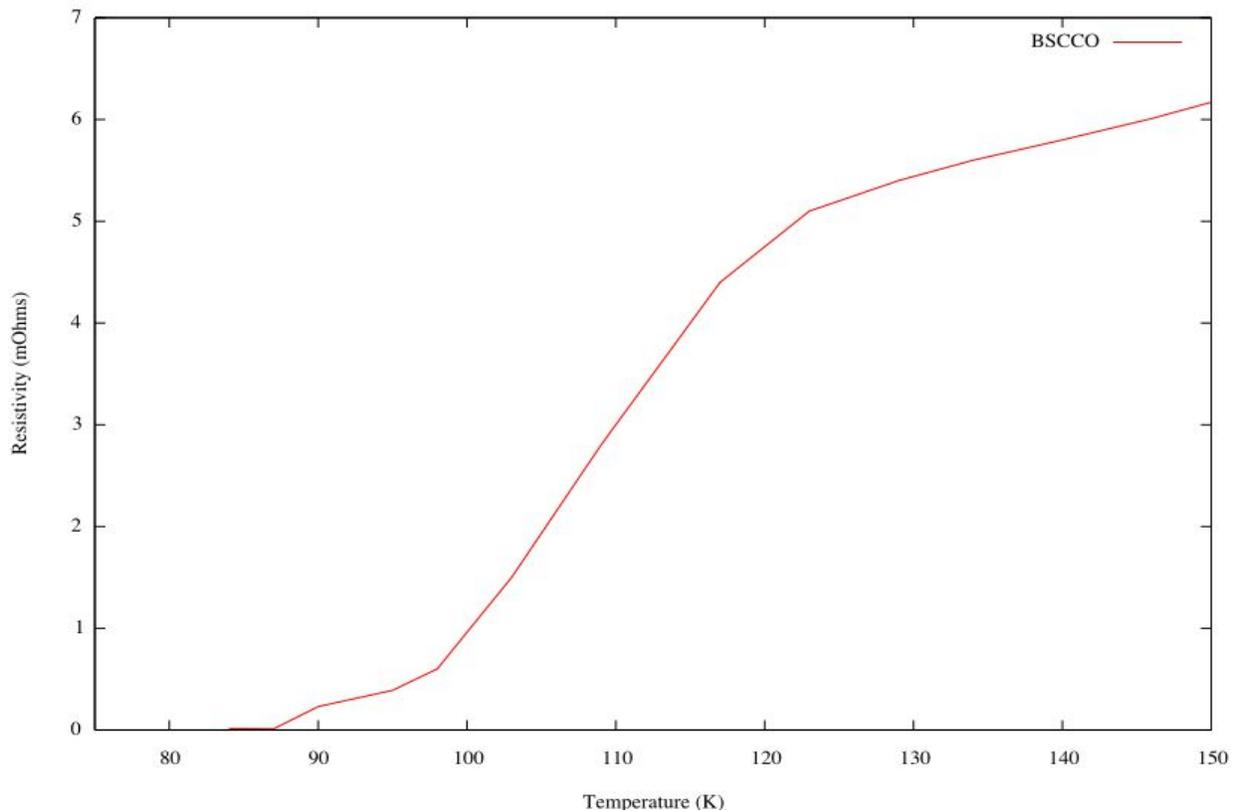
Like many materials, BSCCO's resistance decreases as it cools. Around 100° -120°K, it drops rapidly and under 90 °K, it is too low to measure accurately in this setup.
